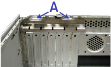
Figure 4 - 23 : Metallic Bracket Tabs
